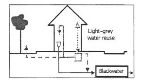
These systems are usually closed systems that collects greywater from shower and bathroom basin within an underground tank where the water is disinfected using continuous UV before re-use for toilet flushing and external garden watering. Storage tank volumes need to be optimised depending on the reuse intention.
